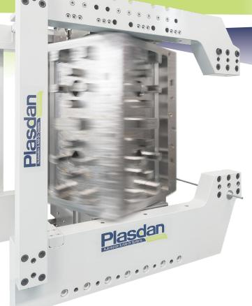
A specialized mold design that enables multi-sided or multi-component injection within a single mold cycle. Cube molds allow for more complex part designs, reduced cycle times, and integrated assembly processes, making them particularly useful for multimaterial or multi-color applications.
